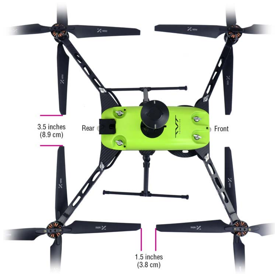
Figure 1. Proper distance between propeller tips
