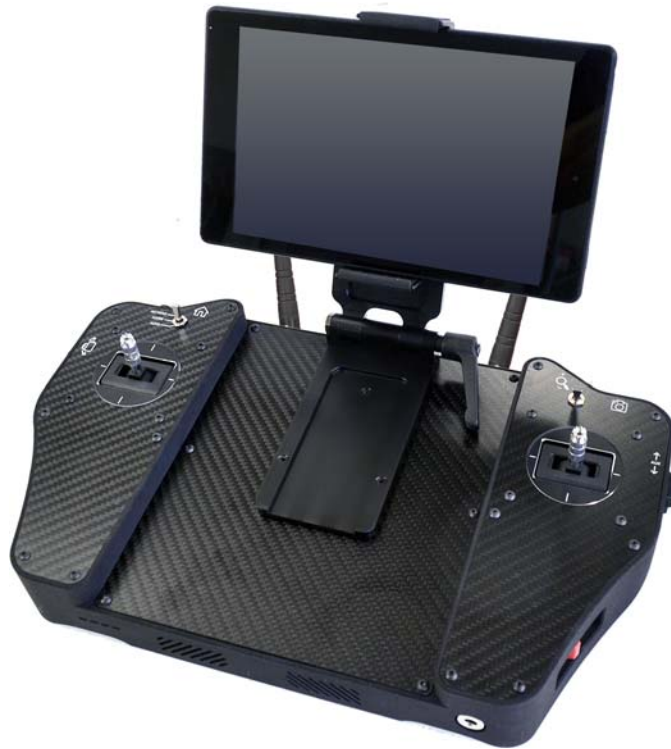
Figure 38. Mounting the tablet on the tablet holder
