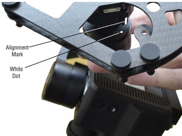
Figure 28. Installing gimbal on gimbal ring
