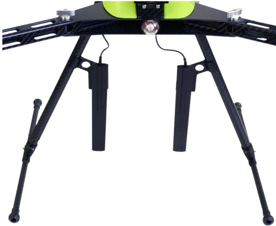
Figure 12. Attaching antenna clips onto landing legs
