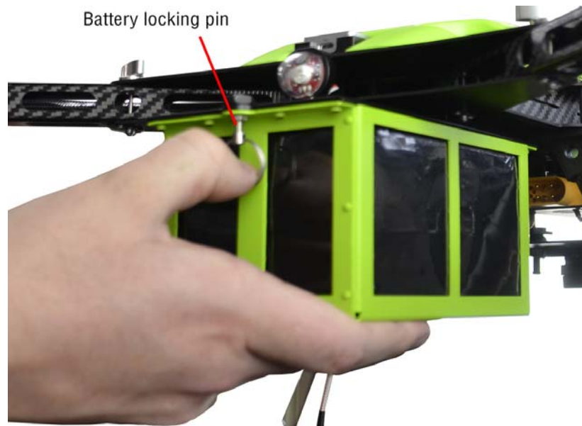
Figure 24. Installing the battery into the airframe rails
