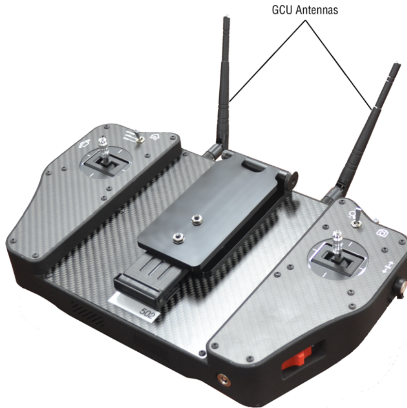
Figure 31. Installing antennas on the GCU
