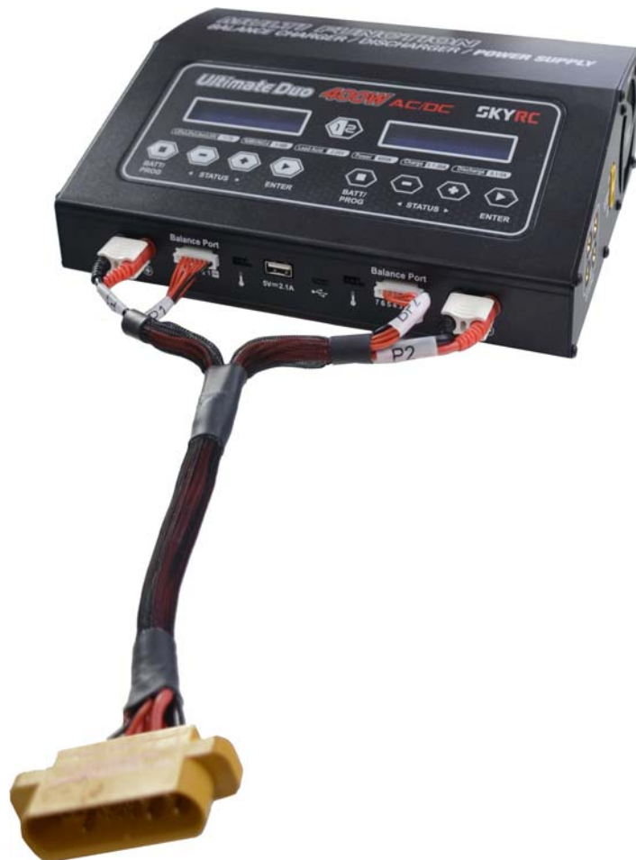
Figure 54. Connecting the battery charging cable to the battery charger
