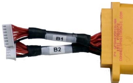
Figure 20. Battery tester cable
