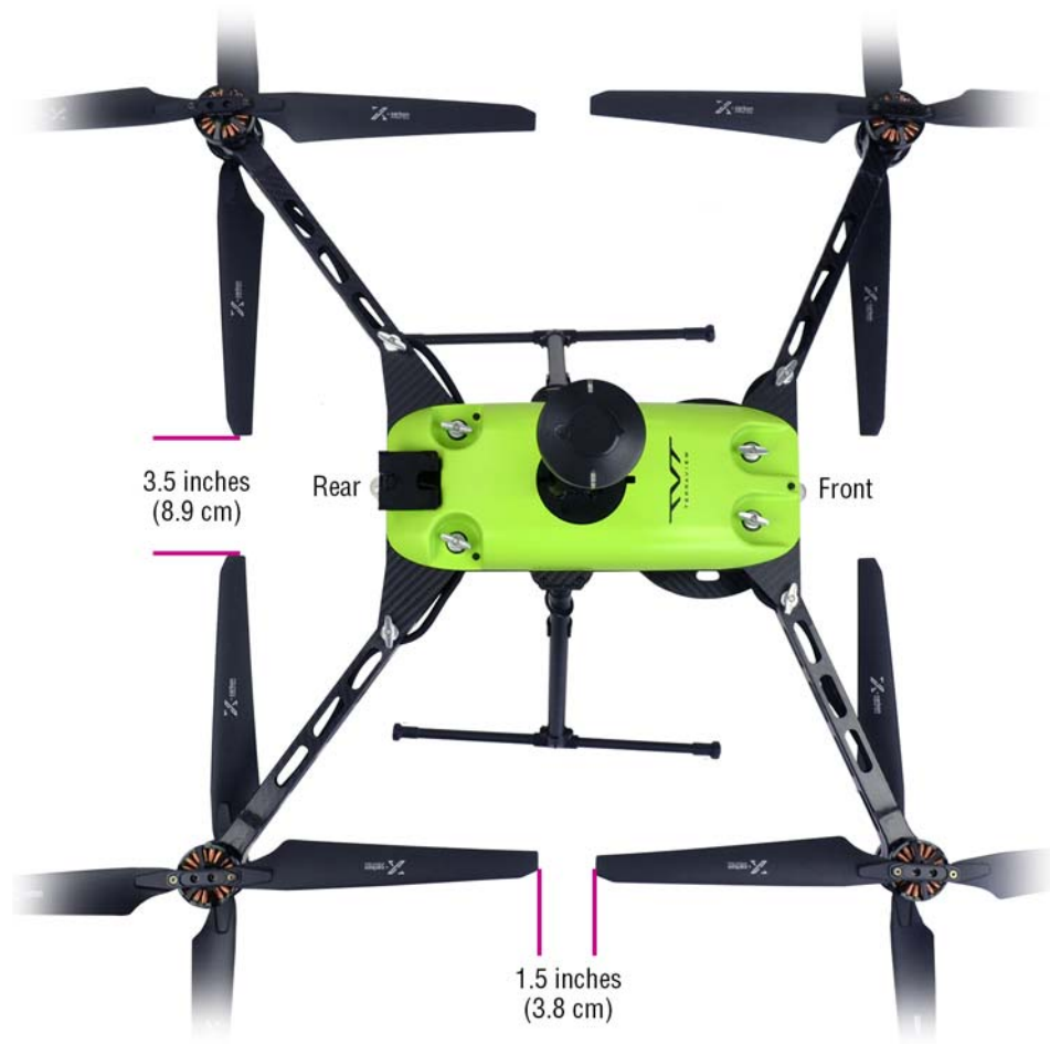
Figure 41. Proper distance between propeller tips
