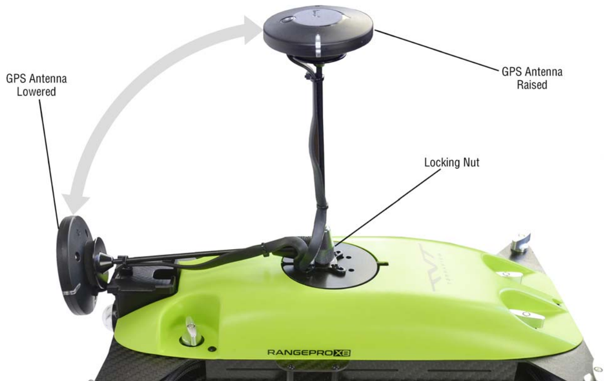
Figure 14. Raising the GPS antenna
