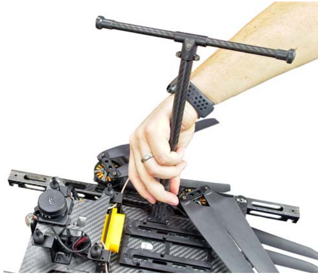
Figure 9. Installing a landing leg
