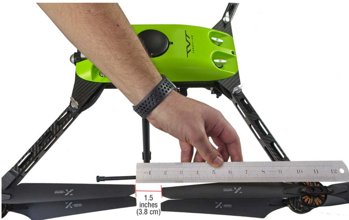
Figure 30. Proper distance between propeller tips
