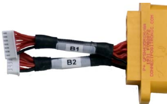
Figure 15. Battery tester cable
