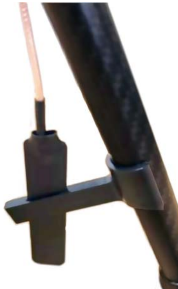
Figure 8. Attaching an antenna clip onto a landing leg
