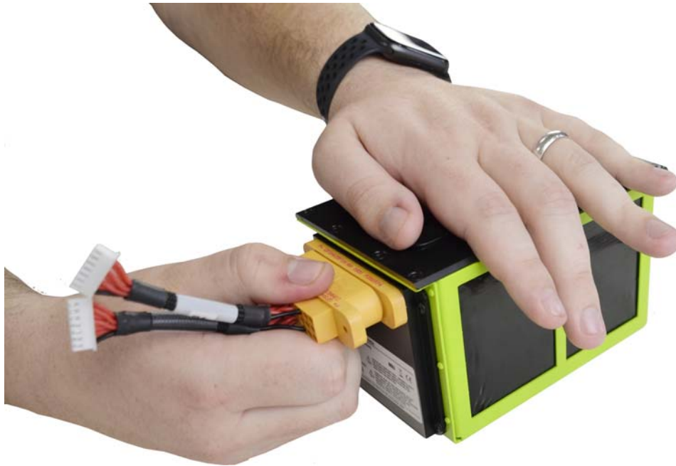
Figure 18. Disconnecting battery tester cable
