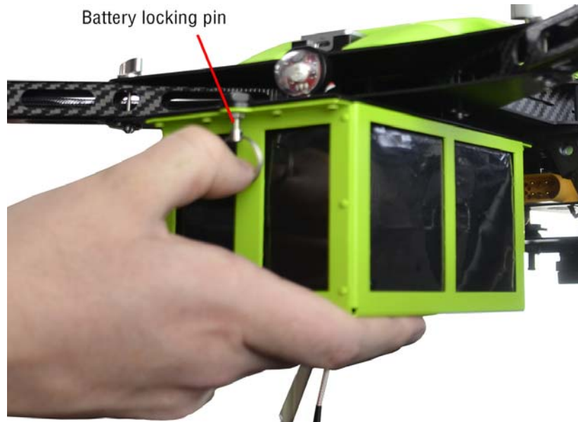
Figure 19. Installing the battery into the airframe rails
