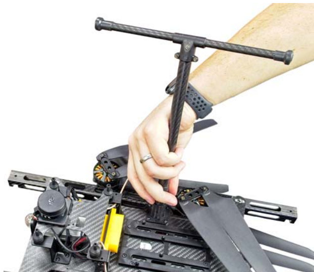
Figure 6. Installing a landing leg
